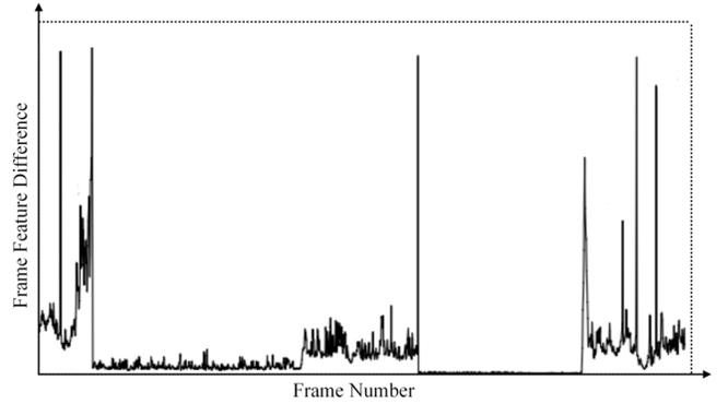
**Figure 4: Frame Feature Deviation** - Plot of  $\psi$  from Equation 3 for frame-frame feature changes. The spikes show abrupt pose changes within the animation (e.g., trips and sudden impacts). The information also provides a visual means for searching for changes when browsing an animation libraries.
