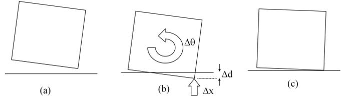
Figure 1. **Penalty Correction** - Corrective position and orientation penalty.
