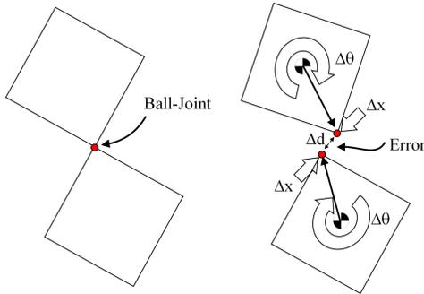
Figure 2. **Joint Constraint** - Connecting relative rigid-body offsets.
