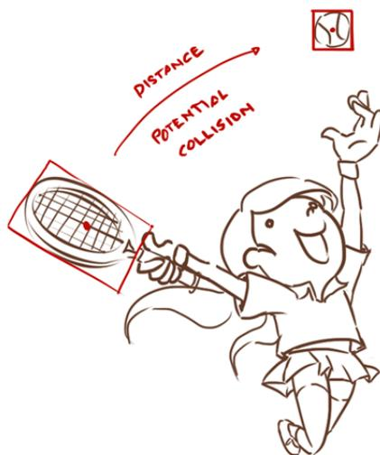
**Figure 1. Narrow Phase** - In broad phase, the task is to avoid performing expensive computations for bodies that are far away from each other. Simple bounding boxes can be placed around each of the bodies, and simple tests can be performed to avoid costly collision checking unless the boxes overlap.
